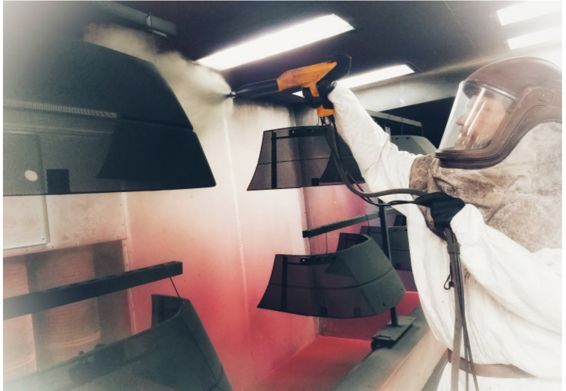
Photo: Powder Coating Booth
